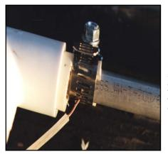
Figure 2—Use hose clamps to secure the aluminum tubing to the PVC T and to attach the coax conductors.
